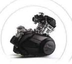
500 H.O. 4-VALVE, SOHC, EFI 38 HP, liquid cooled, single cylinder, 4-valve featuring Bosch® Electronic Fuel Injection and CVTech clutches
